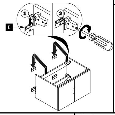
Attach the wall brackets (E) to the wall with the screws (F).
